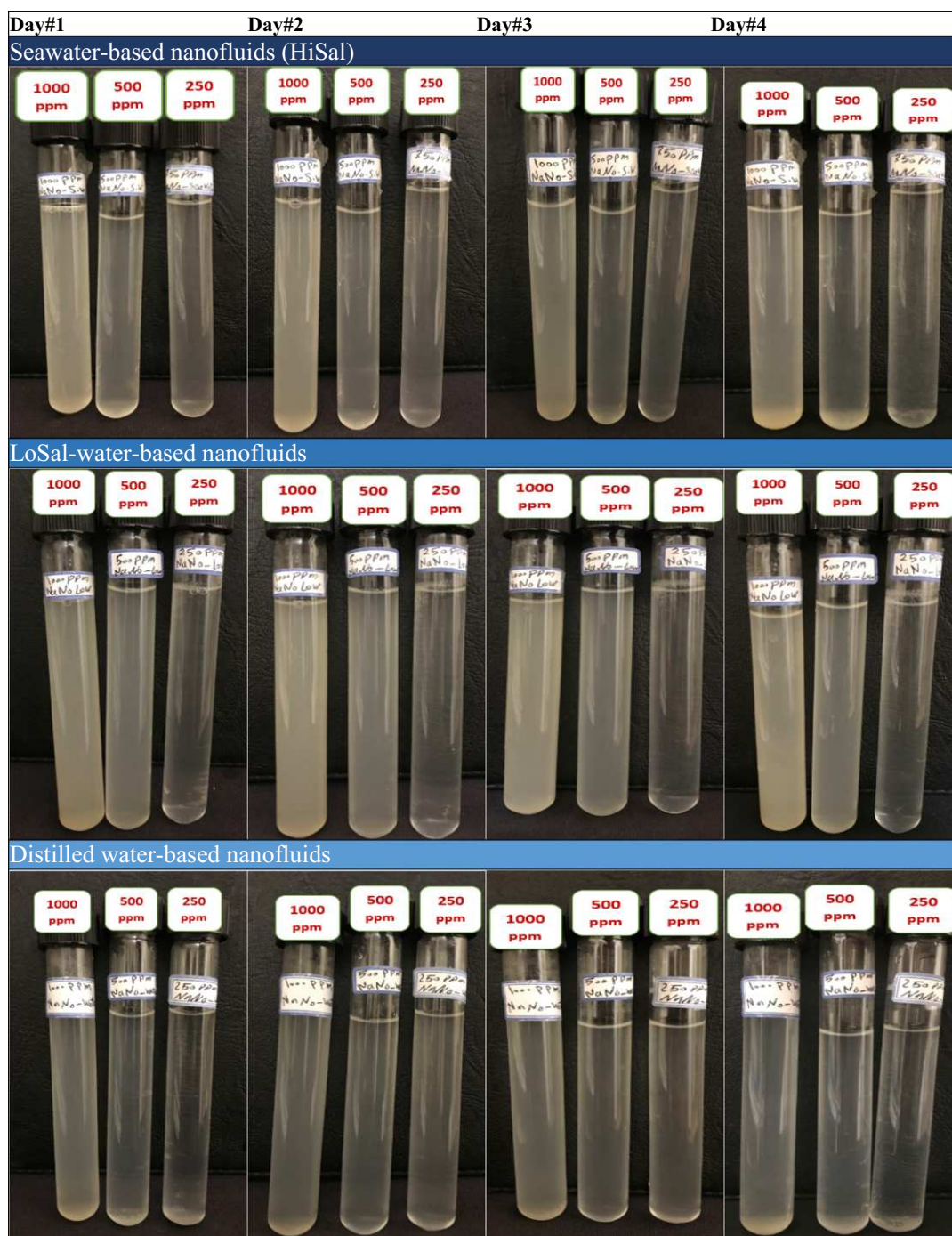
Fig. 11. Dispersion stability of HiSal, LowSal and DW nanofluids w/ NCs concentrations of (a) 250 ppm, (b) 500 ppm, and (c) 1000 ppm after four days.
