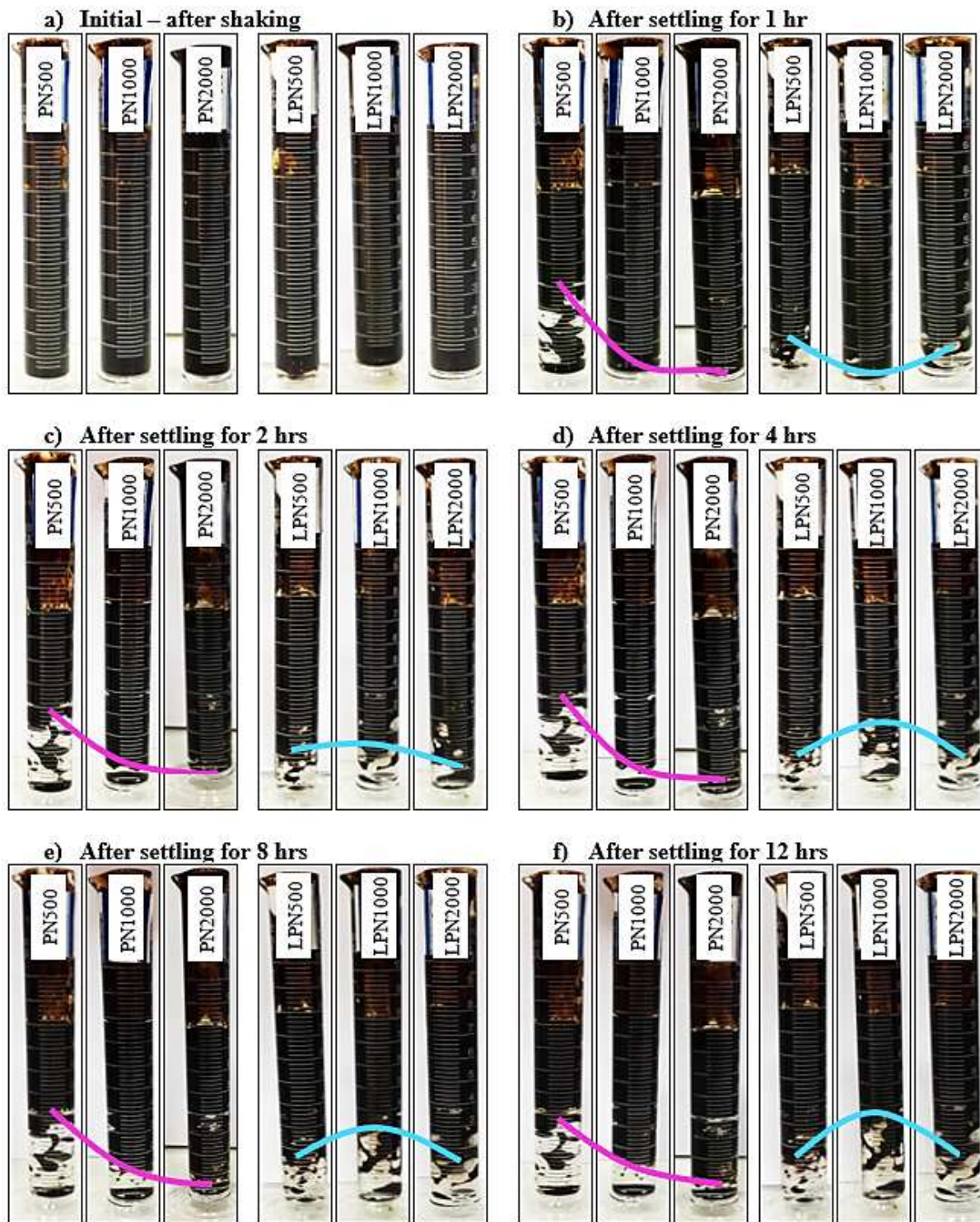
Figure 35 Emulsification images of oil/polymeric and oil/low salinity-polymeric nanofluids over various time-steps.
