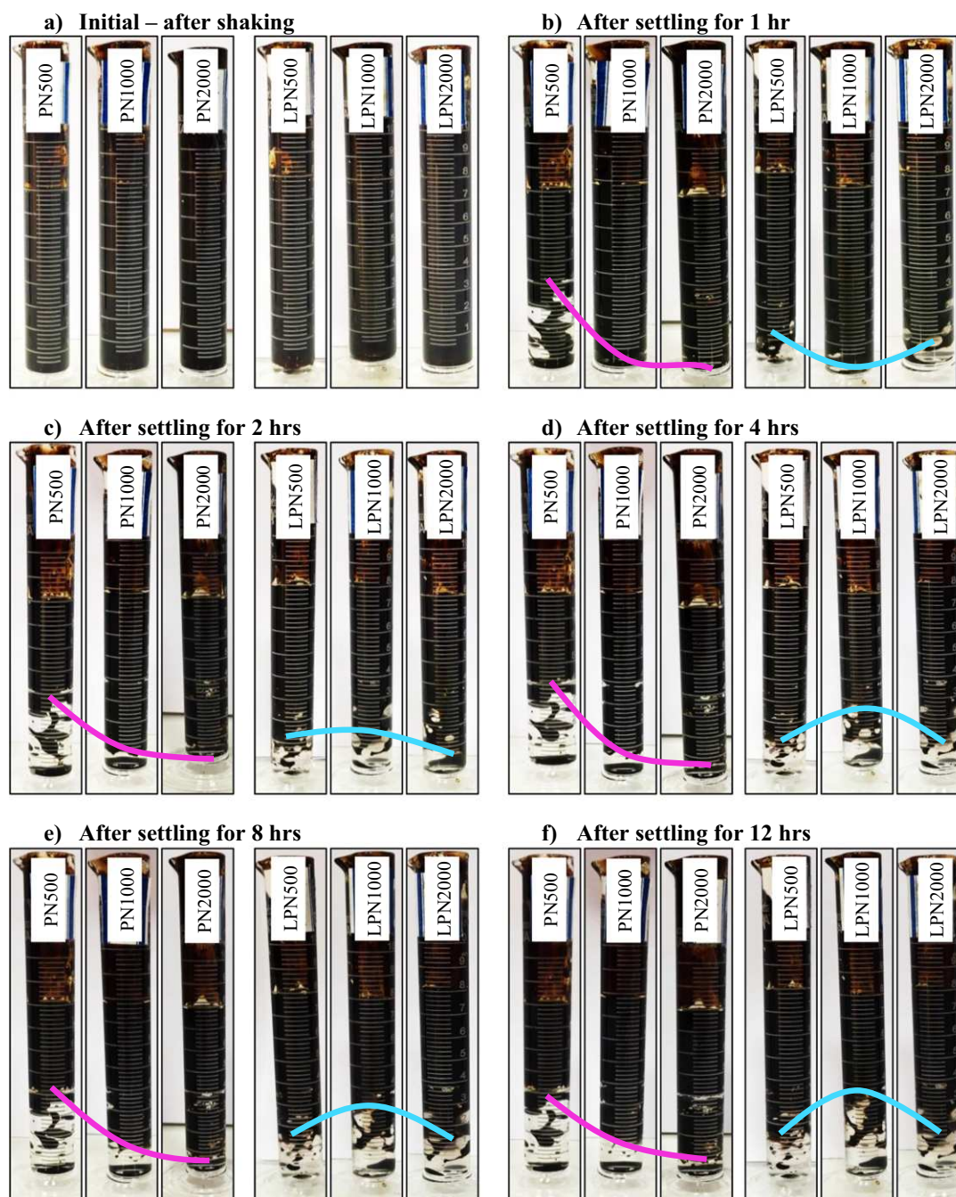
Fig. 15. Emulsification images of oil/polymeric and oil/low salinity-polymeric nanofluids over various time-steps.
